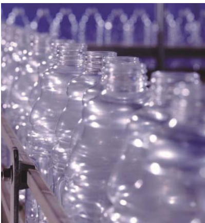
Assist blow for PET bottle transfer
